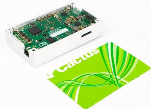
*Picture of the Modem prototype developed by EmTroniX to give users access to the OQ Technology constellations.*
